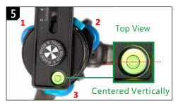
Adjust roller **3** to center the bubble vertically. If this fails due to poor initial leveling, adjust rollers **1** and **2** simultaneously till the bubble is centered horizontally and vertically. Then lock the level locks to prevent accidental change of level.
