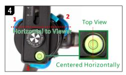
Stand in a position so that 2 rollers (1 and 2) are horizontal in front of you. Look at the bubble from vertically above. Adjust the horizontal rollers to center the bubble horizontally.
