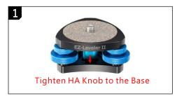
Place the tripod legs in their preferred positions. Tighten the HA Knob to the base. Tighten EZ-L II to tripod while holding the knob with fingers. Then mount the pano head on top of EZ-L II. Mount the camera on pano head.
