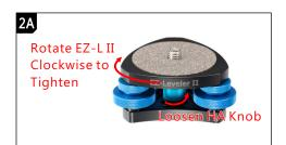
Loosen EZ-L II a bit to help loosen HA Knob. Gradually loosen HA Knob while tightening EZ-L II, until the camera is about to point at the desired direction. Tighten EZ-L II fully. Then continue the leveling process described in the previous section.
