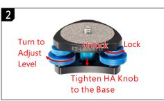
Place the tripod legs in their preferred positions. Unlock the level locks. Turn the rollers to roughly the middle of their full adjustment range. Tighten the "Head Alignment Knob" (HA Knob) of EZ-L II to the base. Tighten EZ-L II to tripod while holding the knob with fingers.
