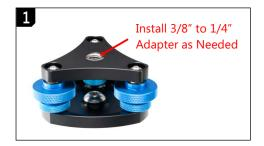
Install the 3/8" to 1/4" adapter if the tripod has a 1/4" thread. If tripod top plate has bare metal surface, consider adding a friction material to prevent loosening and/or scratching the base of EZ-L II. An optional cork sheet like that on EZ-L II is available from Fanotec.
