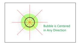
With a properly leveled circular bubble level, the bubble is positioned at the center of the vial. The bubble is horizontally centered when a viewer looks at the center of the vial from any direction. Therefore it suffices that the viewer reads the bubble from any 2 perpendicular vertical planes
